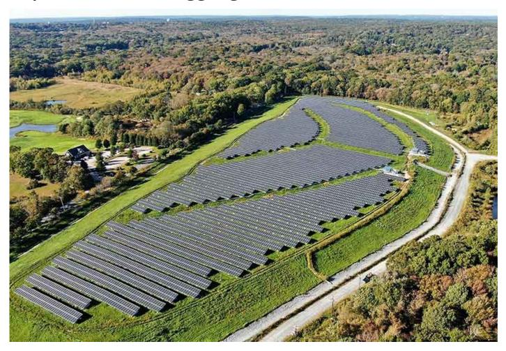
Kearsarge Energy built a 4.7-MW solar project on the Rose Hill Landfill Superfund site in Rhode Island, with engineering design, permitting and construction support by GZA.
