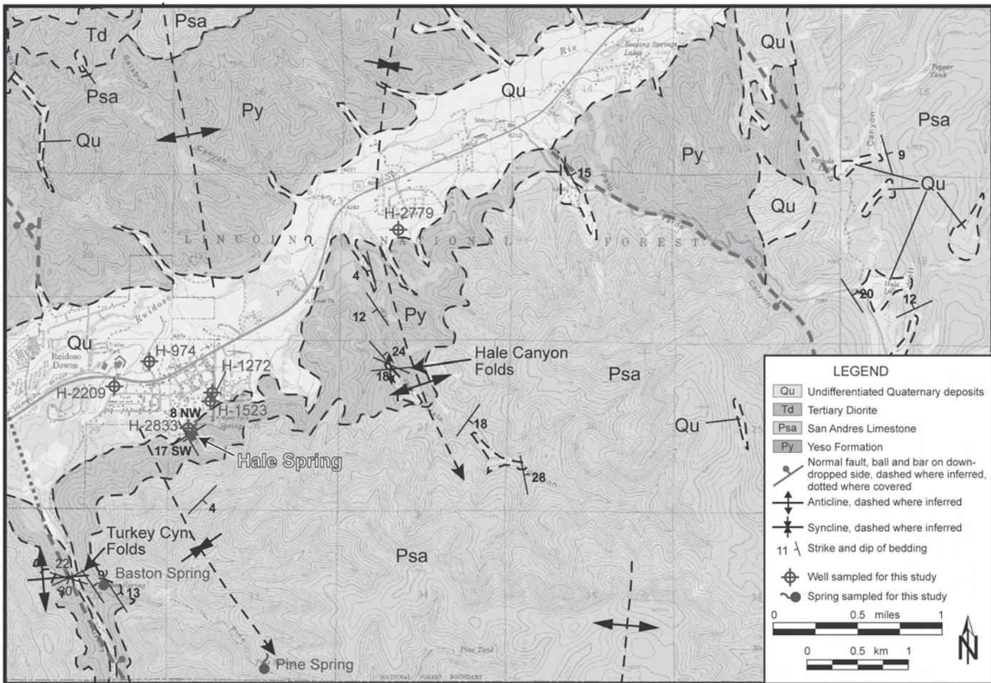
FIGURE 2. Geologic map of area around Hale Spring showing wells and springs sampled for this study. Map compiled from Kelley (1971), Rawling (2004b) and field work conducted for this study.
