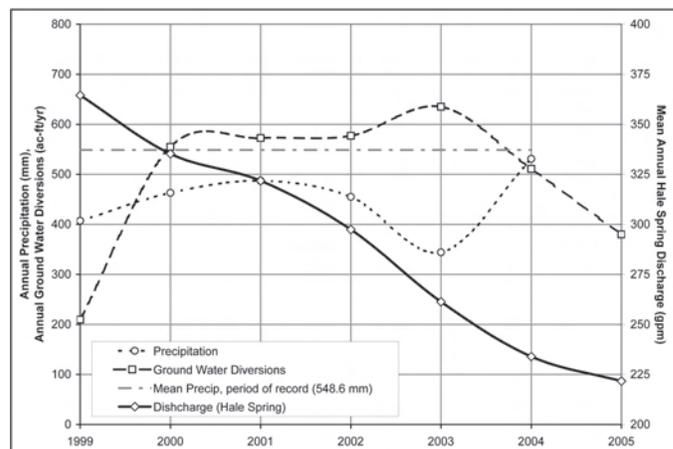
FIGURE 6. Graph of Hale Spring discharge, precipitation, and groundwater diversions from 1999 to 2005.
